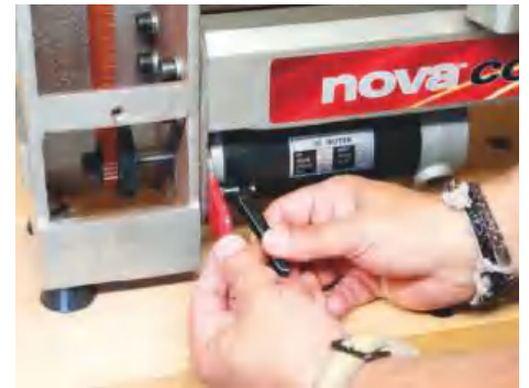
▲ This lever and handle combination is used to swap the belt position
